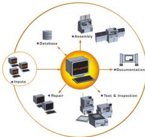
The MPM application enables Autron to unify and integrate the diverse software solutions currently provided by different machine vendors.
